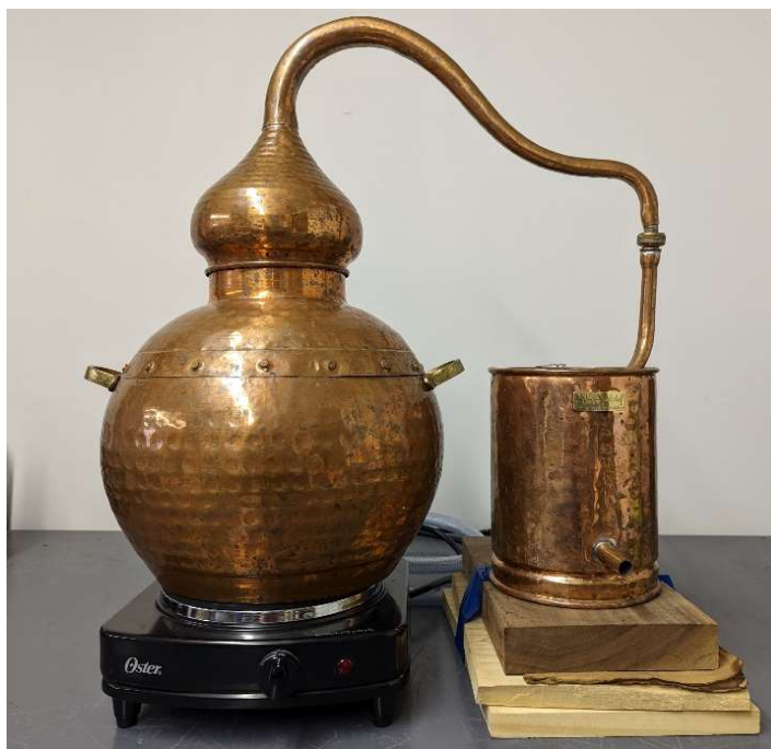
356 357 Figure 7. The 11.36 L (3 US gallon) alembic pot still and hot plate used for all spirit runs. 358
