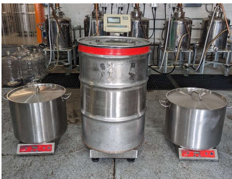
330 331 Figure 5. Equipment setup for weighing fermentation ingredients and heating the water.
