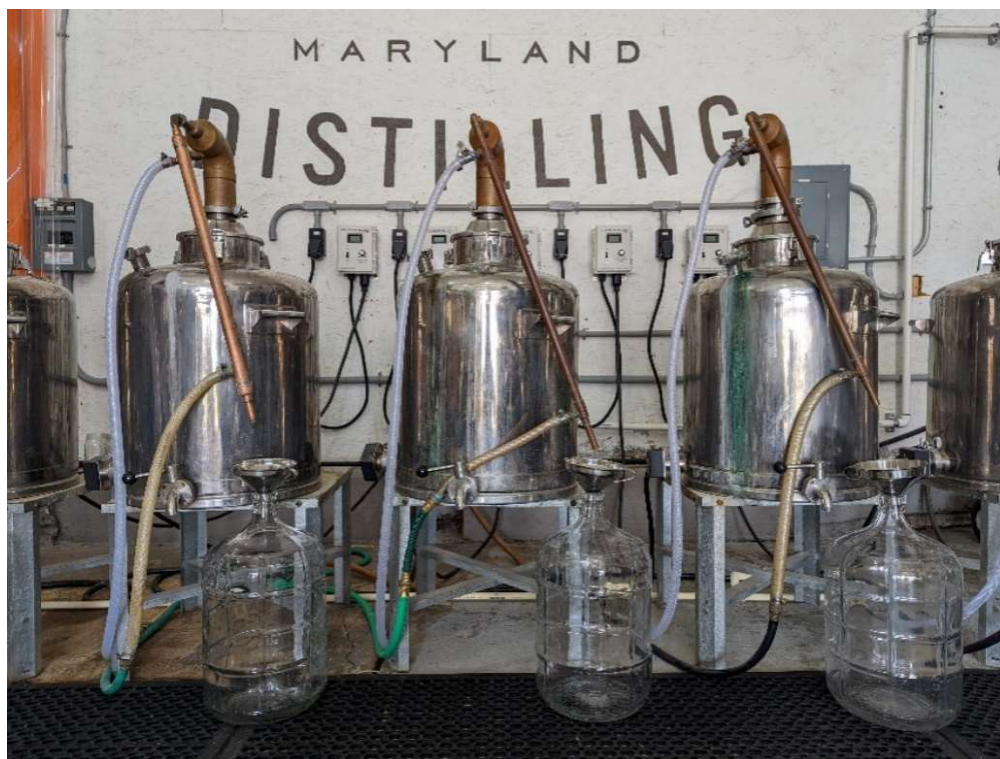
352 353 Figure 6. The 100 L stills that were used for stripping runs, showing controllers and the carboys used 354 for low wines collection.
